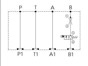
**TECHNICAL DATA** Aluminum Body Pressure Rating: 250 bar Ductile Iron 350 bar **Body Pressure Rating:** Rated flow: 30 I/min
