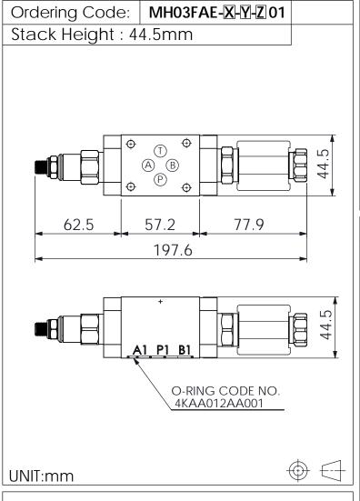
FULLY OPEN RESTRICTOR-FLOW IN BOTH DIRECTIONS
